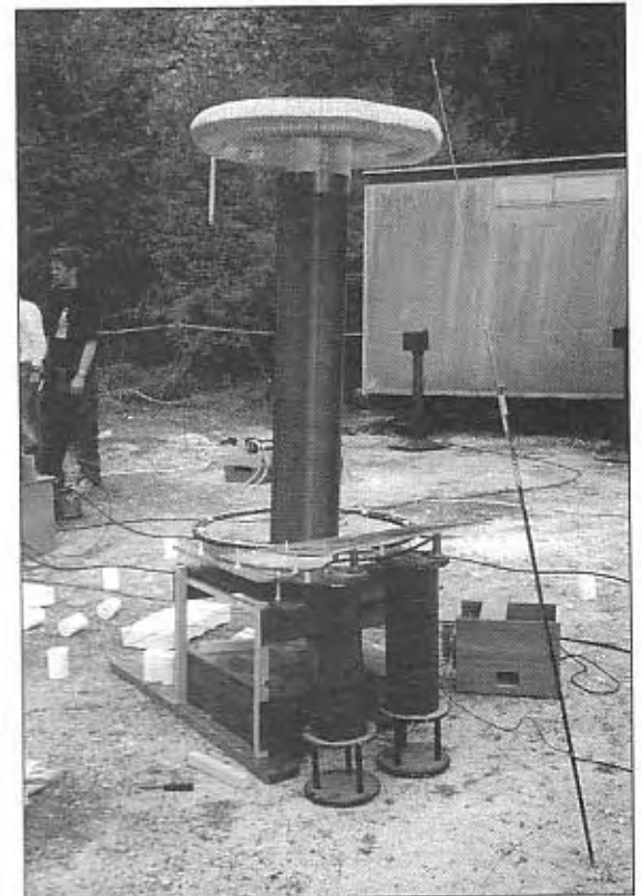
A really big coil. A Tesla coil being set up at Amberley museum. The resonant frequency of this arrangement was around 170kHz.
