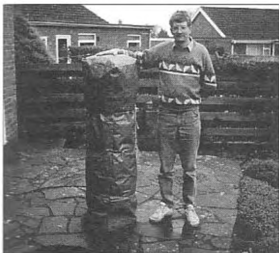
Gift-wrapped. The GW4ALG loading coil with weather protection.
