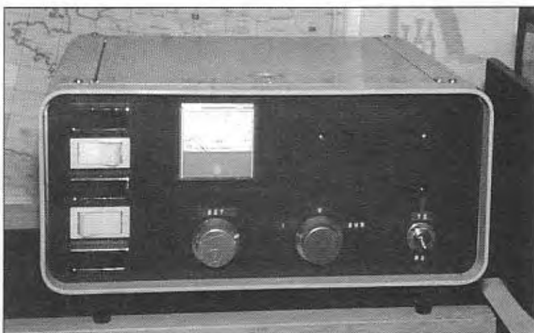
Fig 3.17: General view of the 572B LF transmitter using a converted KW1000 HF linear amplifier purchased for under £200. The original tuning and switching components have been removed and the holes in the front panel blanked over. The original SWR meter and switching has been retained.
