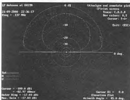
Fig 4.5: Energy distribution of the LF antenna at OH1N. This antenna has a larger horizontal polarisation component than the other antennas.
